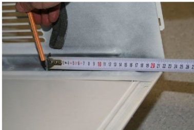
Case and support is bolted to the frame (case-internal dimension 26 cm)
